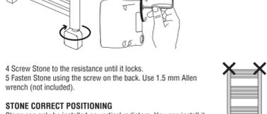
4 Screw Stone to the resistance until it locks. 5 Fasten Stone using the screw on the back. Use 1.5 mm Allen wrench (not included).
